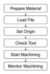
Place the material on the worktable and secure it using vacuum or clamps.
